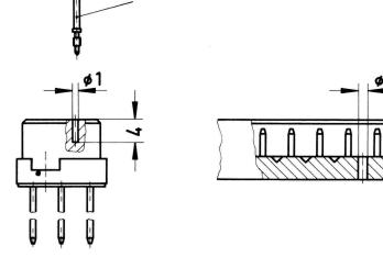
To avoid cross-plugging of adjacent connectors a coding system is required.
