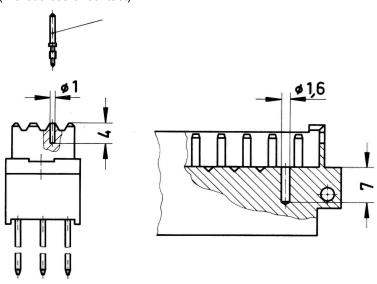
To avoid cross-plugging of adjacent connectors a coding system is required.
