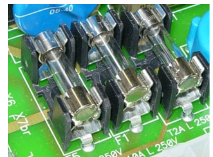
Fig. 2: Fuses mounted in holders and placed so close together as shown can influence each other reciprocally with regard to temperature.
