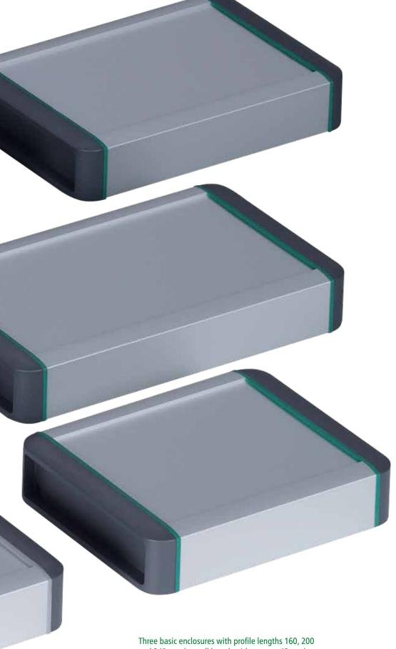
Three basic enclosures with profile lengths 160, 200 and 240 mm (overall length with covers +42 mm), enclosure width 170 mm. Designer seals available in green or volcano grey. Individual profile lengths to customer specifications on demand.
